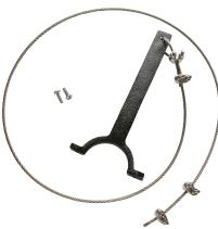
Safety Cap Kits are used to convert standard chainwheels to safetywheels. By adding the safety cap kit, there is a secondary attachment to reduce the potential hazard of a falling valve hand wheel. Included in the kit is a safety cap, 5 feet of 7x19 stainless steel wire with 4 stainless steel clamps, and fasteners required to attach the cap to the guide arm.
