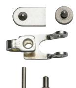
Babbitt Masterlinks are used with weldless chain to connect the two ends during installation of the chainwheel. The Masterlink returns the chain to its original load bearing strength with in a quick and easy process. When a Masterlink is added to an order, the chain is prepared in our facility to eliminate the need for cutting or alteration on site.
