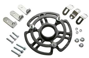
Hammer-Blow Conversion Kits are added to ductile iron chain wheels that are attached to problematic or sticky valves. The "hammer" action makes opening or closing sticky valves easier for an operator of any size without damaging the chainwheel or valve. This accessory can only be added to ductile iron chain wheels because of their shock resistant construction. Included in each kit is the Hammer-Blow mechanism and fasteners required to attach the mechanism to the spokes of the chainwheel.
